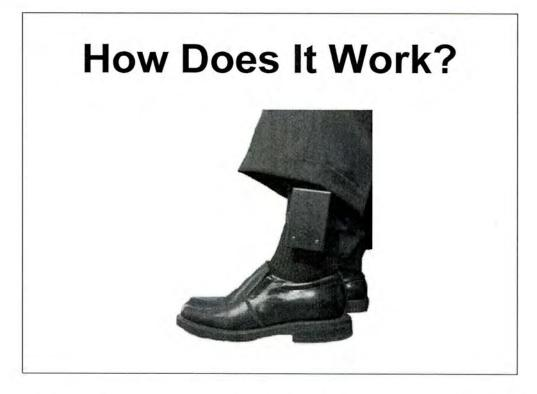
The Stun-Cuff is placed on an individual's ankle or wrist. The Activator is a remote trigger that provides a high voltage, low amperage stun to the wearer. This stun is similar to the effect of a stun gun and gives an initial stun of 2-3 seconds. The Activator can allow for a longer stun as needed and this stun can be given from distances up to 100 yards.
